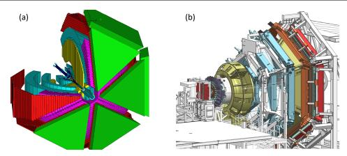
Fig. 3 (a) Model of the original CLAS spectrometer for use with electron and photon beams up to energies of 6 GeV with one of the six sectors removed to enable a view within the detector. The overall length of the detector is  $\sim$ 6 m. (b) Model of the new CLAS12 spectrometer for use with electron beams up to 11 GeV. The overall length of the detector is  $\sim$ 15 m.
