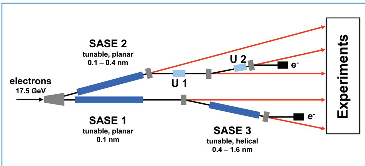
**Figure 4.2** Schematic view of the branching of electron (black) and photon (red) beamlines through the different SASE and spontaneous emission undulators. Electron beamlines terminate in the two beam dumps and photon beamlines in the experimental hall.
