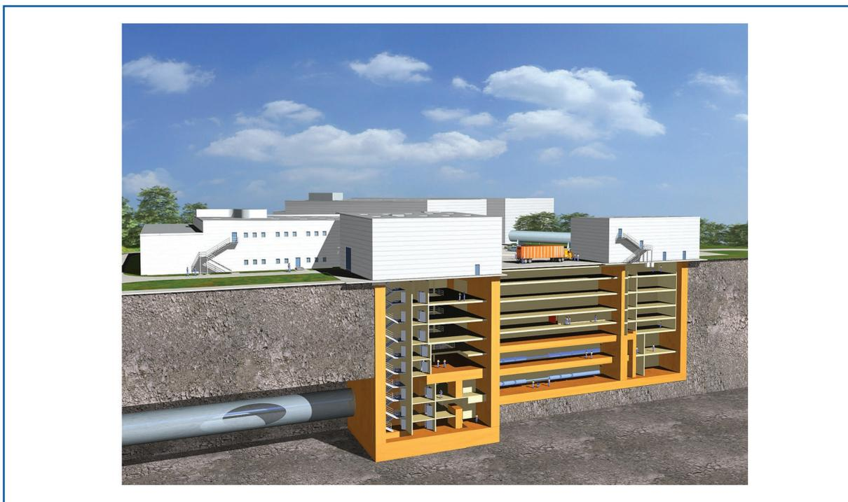
**Figure 7.1.7** Three-dimensional view of the injector complex at the XFEL site DESY-Bahrenfeld.
