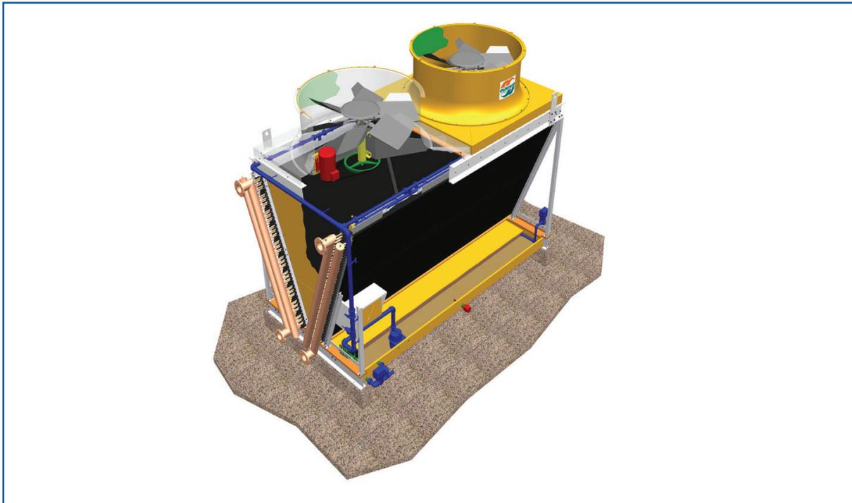
**Figure 7.2.2** Hybrid dry cooler.
