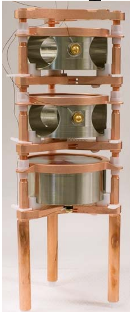
LBNL test string (w/ thermal blanks)
