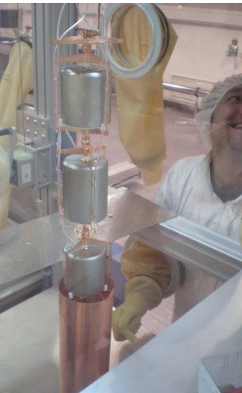
65 \mu m Cu cylinder ('mini-shroud') to shield E-field
