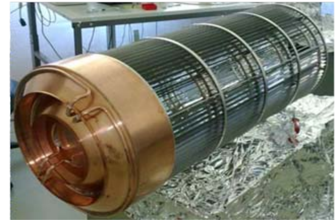
no line of sight between pump and vacuum chamber
