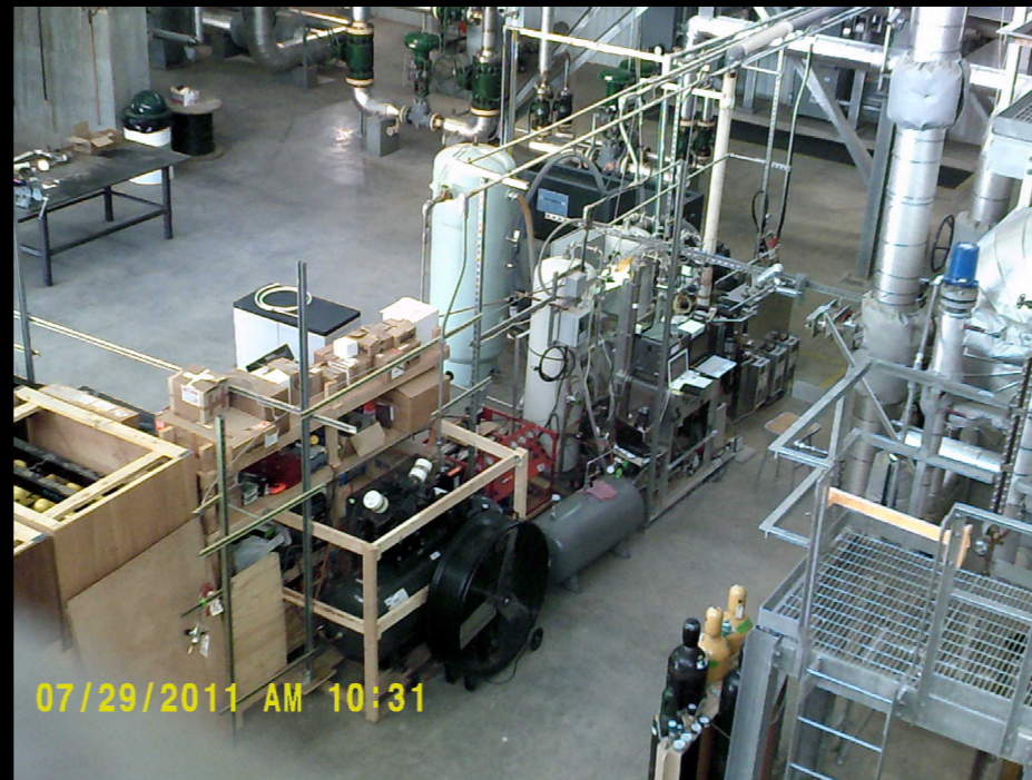
VPSA system (Cortez) 0.5 kg/day production 110 kg produced so far
