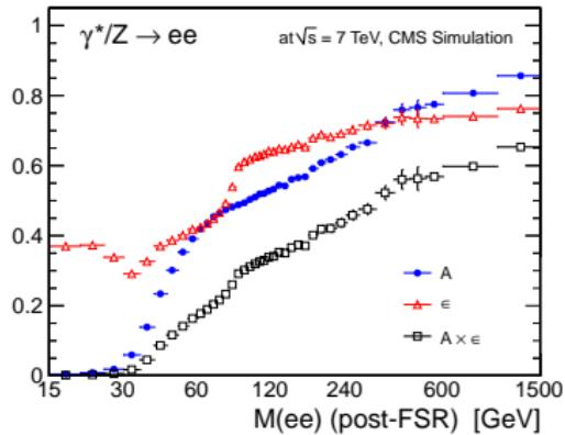
DY acceptance (blue, filled circles), efficiency (red, open triangles), and their product (black, open squares) per invariant mass bin, for the  $\mu^+\mu^-$  (left) and  $e^+e^-$  (right) channels
