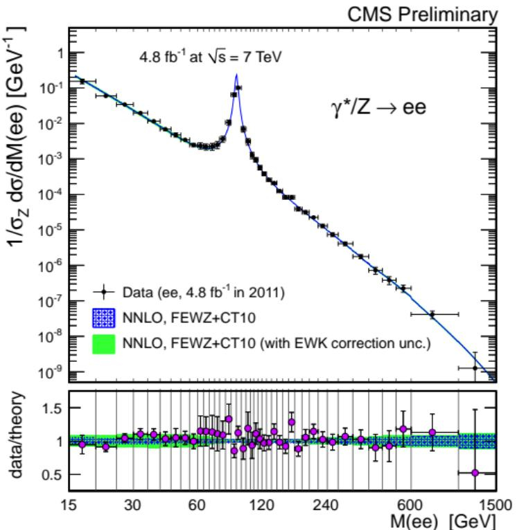
The Drell-Yan invariant mass spectrum in the combined channel, normalized to the Z region,  $r = 1/\sigma_Z * d\sigma/dM$  (NNLO).
