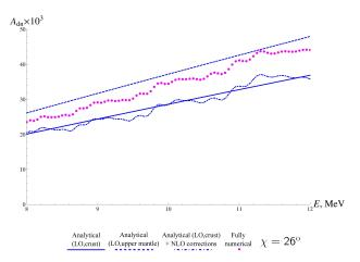
The constant vertical shift is due to the unaccounted fine structure of the crust under the detector. It is smooth enough and is season-independent, so we do not bother about it.
