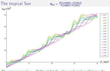
The curves around  $\chi = 23.5^{\circ}$  exhibit the clean and vivid oscillations; the positions of the peaks are very sensitive to  $\Delta m^2$  and  $\{r_{j}\}$
