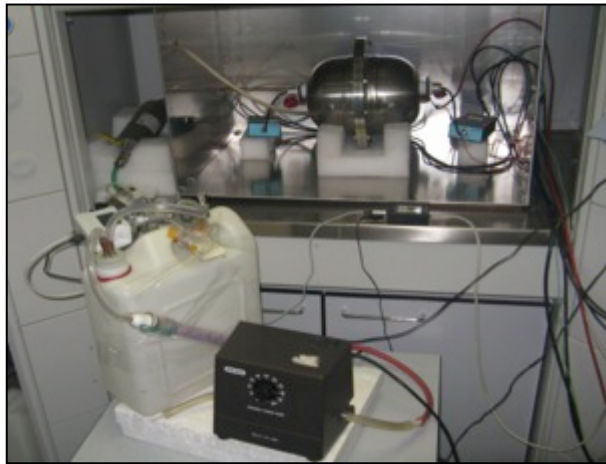
Prague : setup to measure permeability of materials
