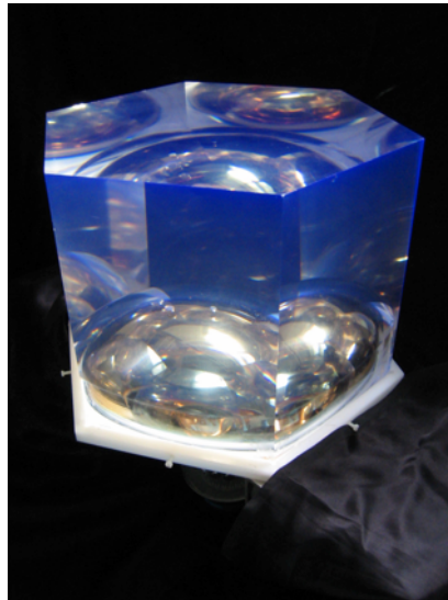
8" PMT + Plastic Scintillator
