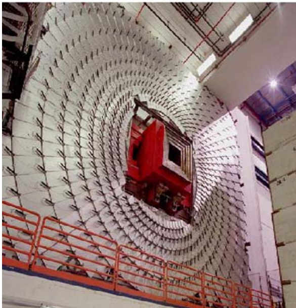
Muon counters plane (6 in total) of D0 experiment (IHEP)
