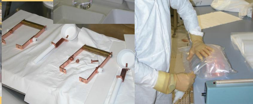
(all operations involving crystals and PMTs -including photos- in HP N<sub>2</sub> atmosphere)
