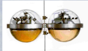
Quasar photodetector ( \varnothing=37\text{cm} )
