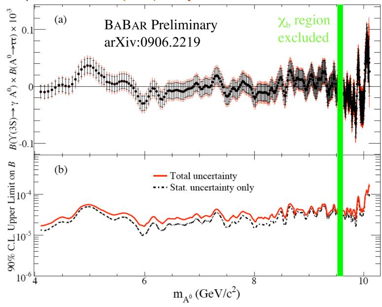
Bayesian 90% C.L. upper limits: significant constraints on NMSSM parameter space Also set a limit  $\mathcal{B}(\eta_b \to \tau^+ \tau^-) < 8\%$
