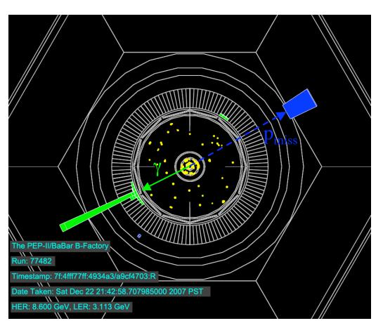
Dominant background from  $e^+e^- \rightarrow \gamma \gamma$ , with one of the photons missing the EM calorimeter. Veto such events by detecting activity in the muon detector (IFR).
