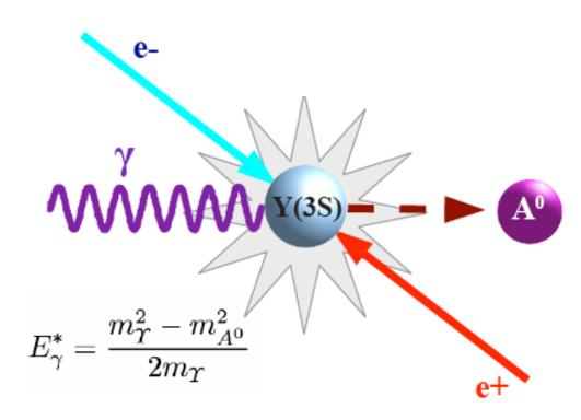
Key experimental signature: monochromatic photon in the Center-of-Mass (CM) frame Well-understood initial state (narrow  $\Upsilon(2S)$  or  $\Upsilon(3S)$  resonance) Fully or partially reconstructed final state, depending on the decay pattern of  $A^0$
