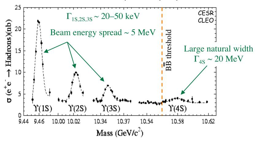
For any bottomonium process  $BF_{nS} = \Gamma_{nS}/\Gamma_{tot} >> BF_{4S}$ , n=1,2,3Significantly better sensitivity to new physics @ narrow resonances
