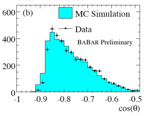
Use data distributions in the polar angle to re-weight the simulated events, recompute efficiency. Plots shown after re-weighting. Correction of 1.088±0.012 (applies to the product of efficiency and BR( $\Upsilon(3S) \rightarrow \pi^+\pi^-\Upsilon(1S)$ )
