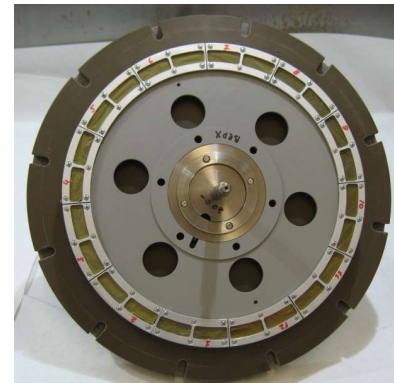
^{242}\text{Pu} 24-cm target wheel 12 sectors
