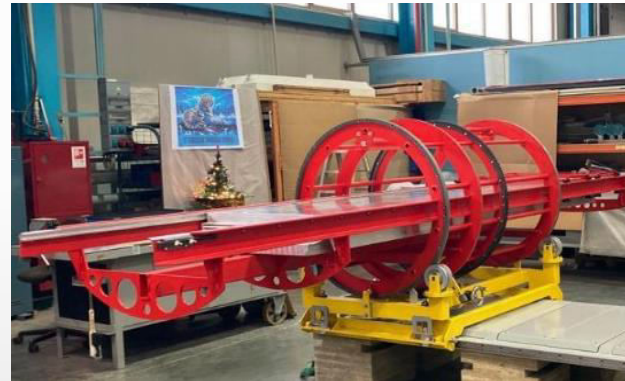
TOF installation bench in LHEP
