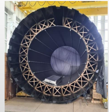
Carbon fiber support frame sagita ~ 5 mm at full load
