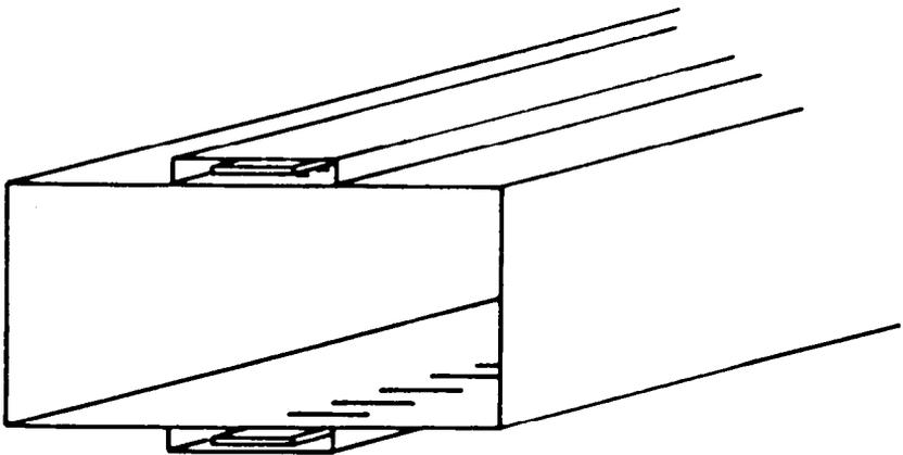
Fig. 10. Slot-type pick-up or kicker. One end of the transmission line is terminated with its own characteristic impedance.
