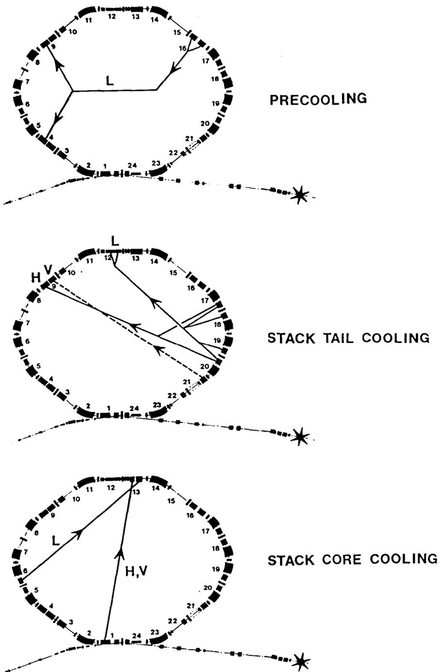
Fig. 14. Plan of the AA ring with its 7 cooling systems. L = longitudinal, V = vertical, H = horizontal.
