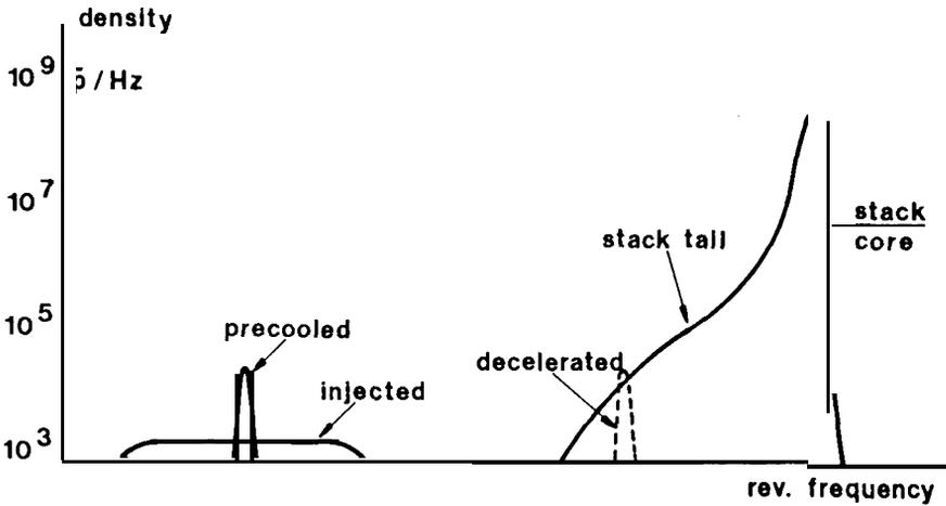
Fig. 11. Density distribution vs. revolution frequency in the Antiproton Accumulator. On the right, the stack; on the left, the newly injected batch, before and after precooling.
