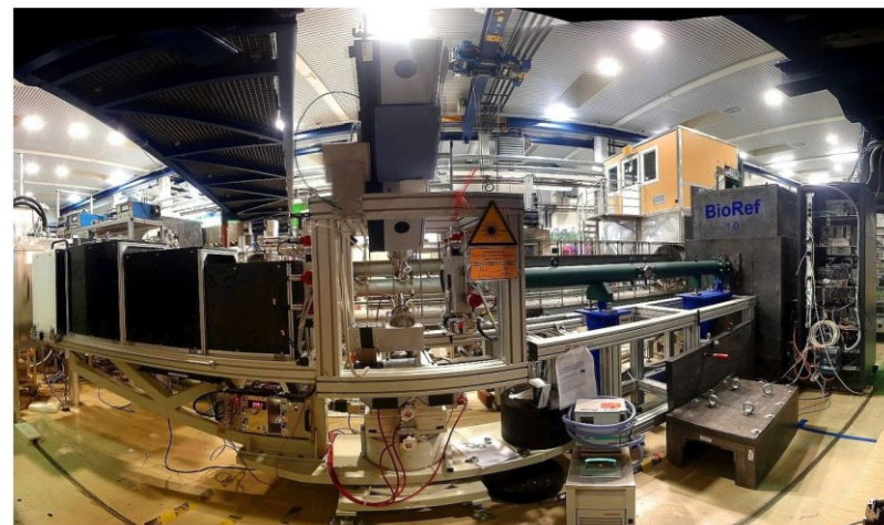
A fish-eye perspective of the new BioRef neutron reflectometer at the neutron source BERII at the Helmholtz Zentrum Berlin with the sample position in the center. The neutrons are guided through a chopper system from the right side and are detected with a position sensitive detector on the left side. As a special feature an infrared beam line is installed on the sample stage, with an infrared spectrometer on top, in order to perform combined infrared spectroscopy and neutron reflectivity measurements. The software
