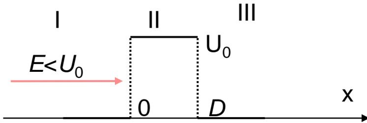
$$-\frac{1}{2} \frac{\partial^2}{\partial x^2} \varphi(x) + V(x)\varphi(x) = E \cdot \varphi(x)$$
