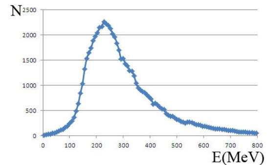
$E_\gamma$  energy spectrum from all partial channels
