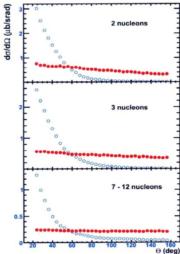
Figure 6: Measured angular distributions of nucleons produced in photodisintegration of  $^{12}\text{C}$  in the laboratory system in events with two (top panel), three (middle panel), seven and more fragments (bottom panel). In all cases the angular distribution for the leading most energetic proton in each event is presented by open circles, while the distributions for all other nucleons in the same event are presented by solid circles.
