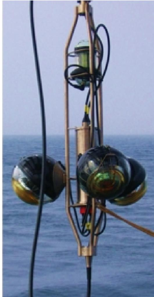
Optical module is a glass sphere with one 10" PMT
