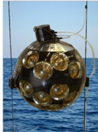
31 x 3" PMTs + electronics in a single glass sphere
