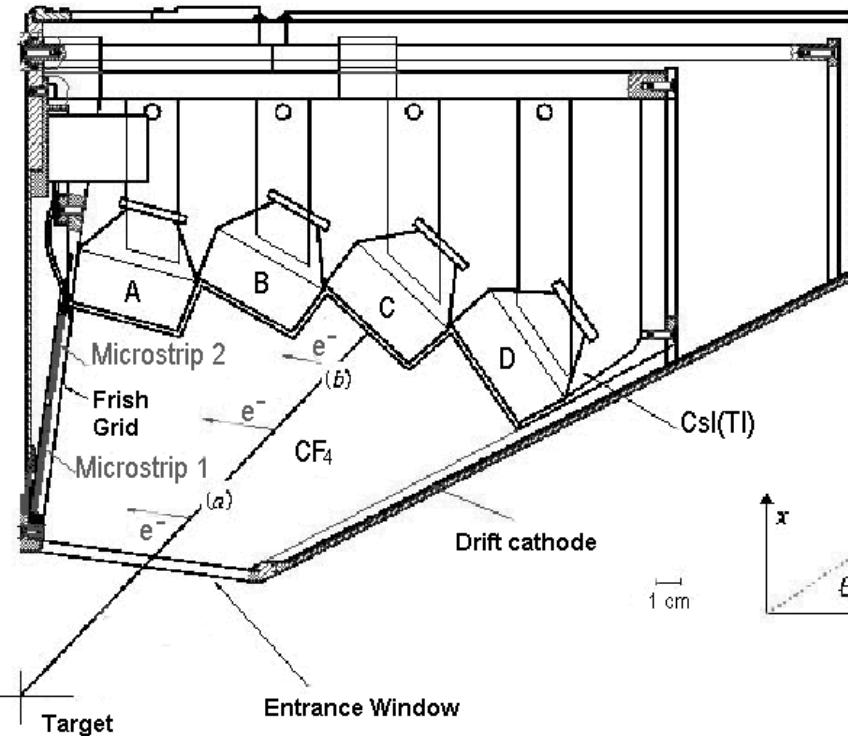
GARFIELD -  $4\pi$  complex multidetector apparatus for particle detection
