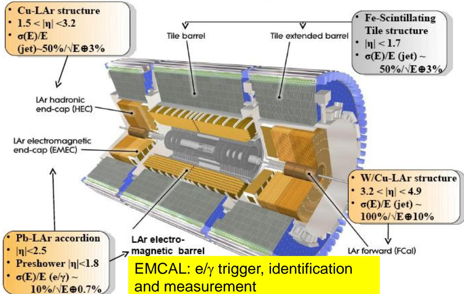
EMCAL: e/ $\gamma$  trigger, identification and measurement
