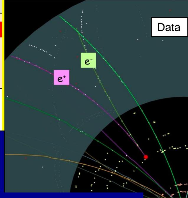
Reconstructed conversion point in the radial direction of  $\gamma \rightarrow e^+e^-$  from minimum bias events (sensitive to  $X_0$ )
