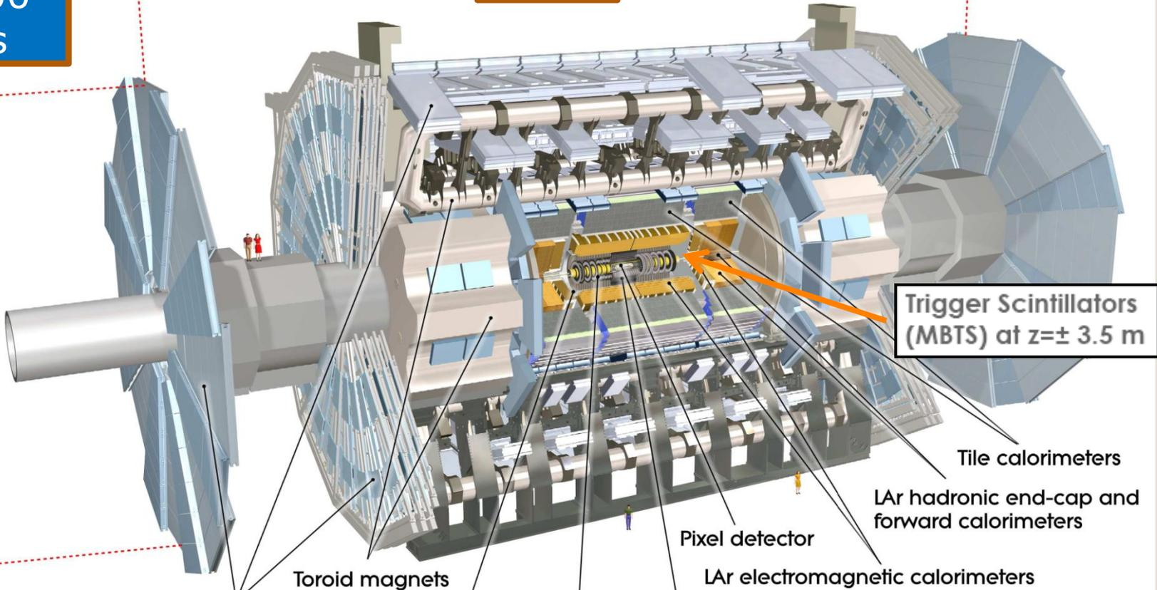
Trigger Scintillators (MBTS) at  $z = \pm 3.5$  m
