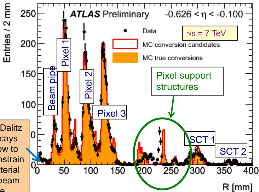
$\pi^0$  Dalitz Decays allow to constrain material in beam pipe
