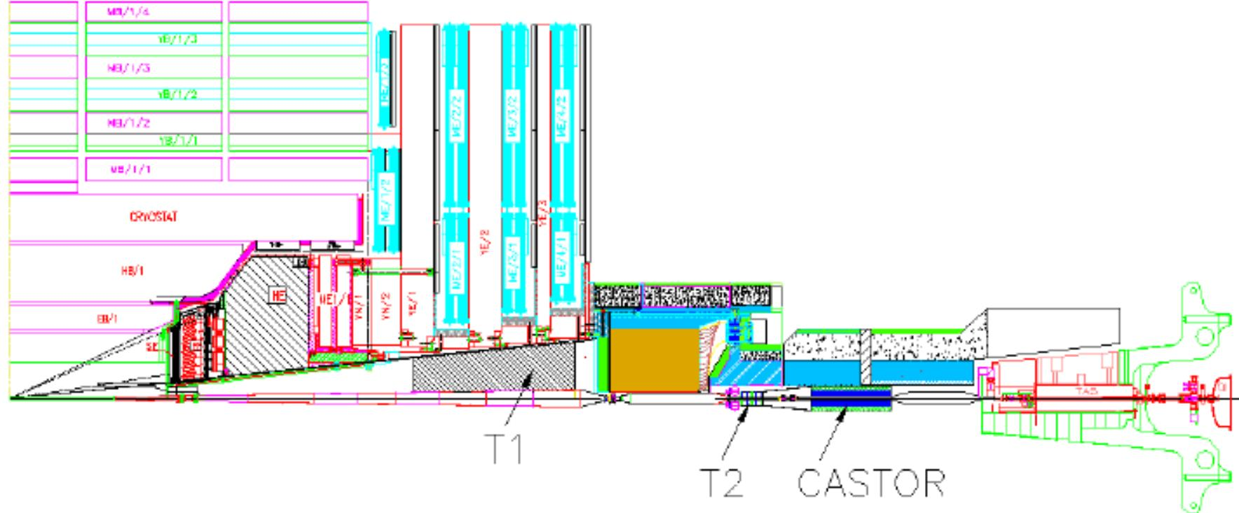
Figure 1.1: The TOTEM detectors are installed in the CMS forward region
