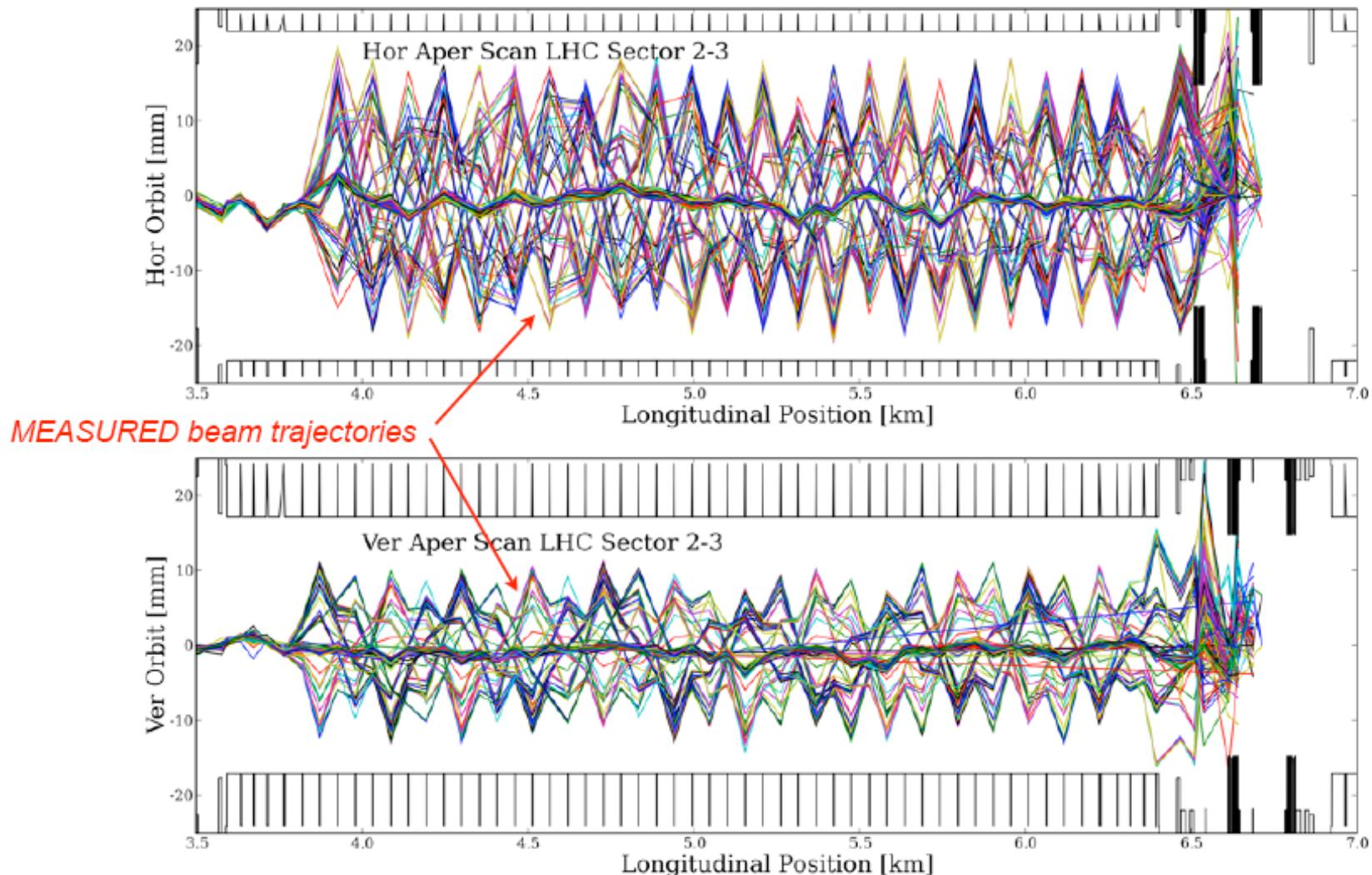
**Horizontal arc aperture of 18-20 mm!!**
