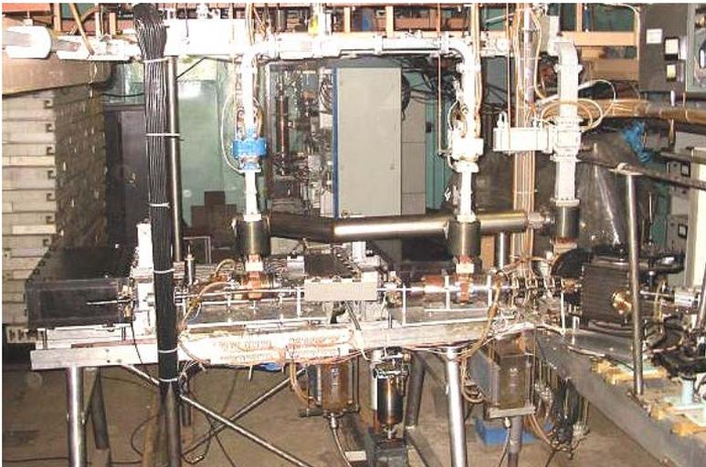
Large dipoles built with rare-earth permanent magnet material, RF gun with photocathode
