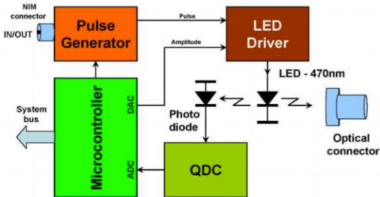
Block diagram of the LED source operation principle
