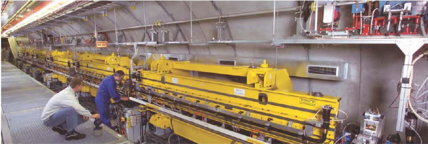
The undulator section in the FLASH tunnel
