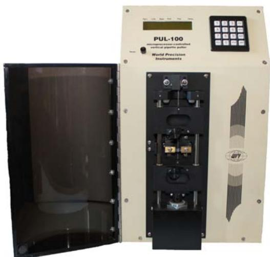
Рис 4. Microprocessor-controlled micropipette puller.
