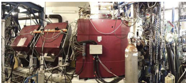
Figure 23. Panoramic view of RITU. The SAGE array for prompt spectroscopy is on the right, where the beam comes from. The optics elements of RITU are from right to left: dipole and two quadrupoles. These elements are preceded by one more quadrupole, not visible in the picture. Part of the GREAT focal plane is visible on the left.
